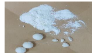
4) 200mg of marrowbone after grinding at 75000 rpm – 10x20s (1 min break)
