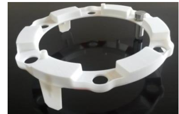
2) Metal tube adaptor (6 samples at once)
